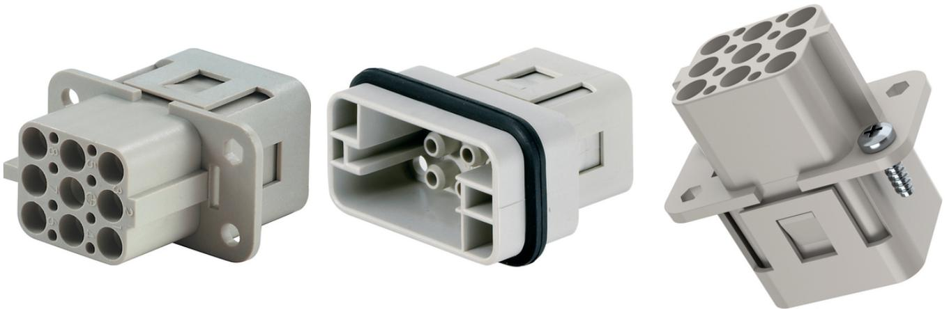
Powerful up to 16 A despite extremely space-saving size for very small devices. Crimp connection creates a vibration-proof connection, ensures maximum contacting reliability between contact and cable and is suitable for automated assembly. Mateable with market standard connectors.
