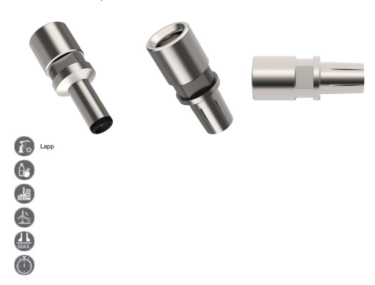
Axial screw contact that can be freely rotated in the high-current module simplifies assembly, prevents torsional stress and thus ensures contact reliability between contact and wire.
